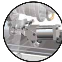
Air-actuated Controls Air shift actuators enable remote operation of band brake and drum clutch, and are standard features for most HP models
